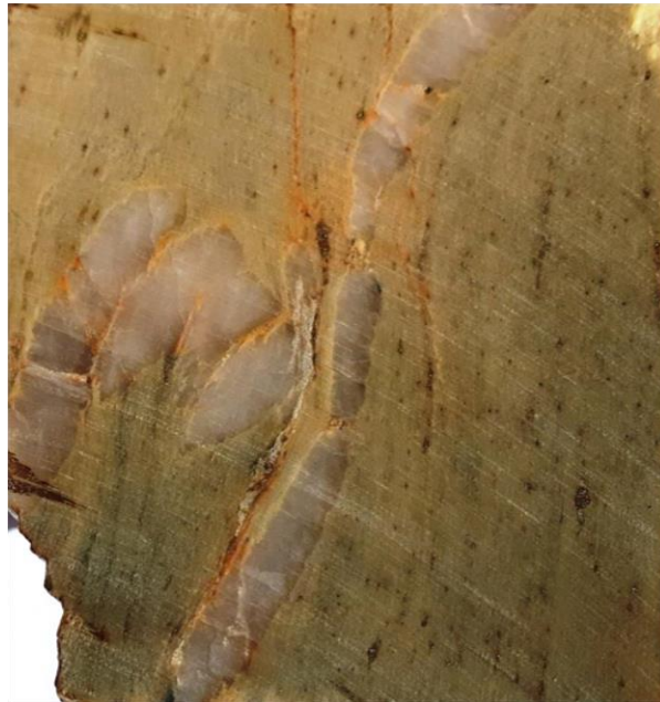
Figure 23-8: Cross-section photo of sawed Porphyry Unit, looking west, containing a P-Zone vein (field of view of Author's photo is 20 cm).
