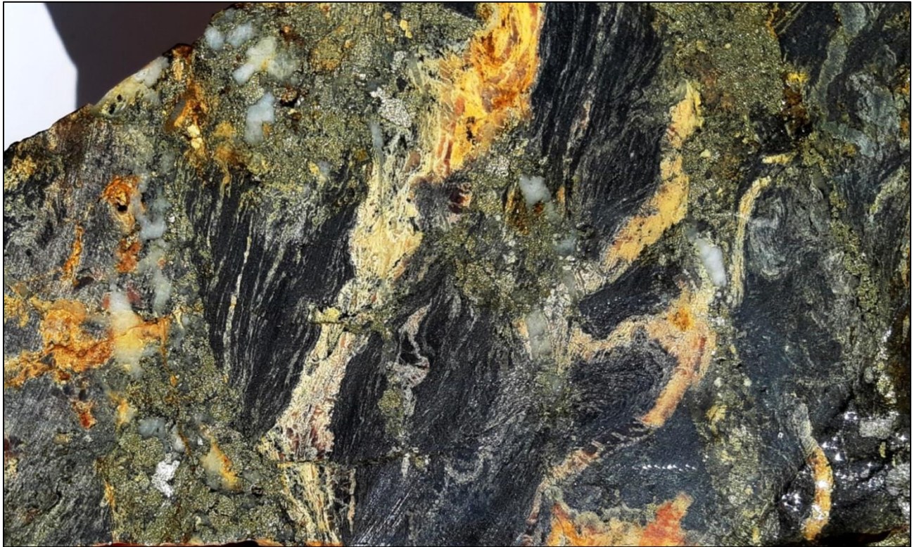
Figure 23-2: Hand sample photo of North Zone Type ore, exhibiting pyrite-quartz replacement of banded magnetite iron formation. K-Zone exhibits similar mineralization. Field of view is about 25 cm. (Author's photo)
